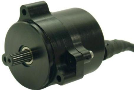
Permanent magnet alternators can tolerate high ambient temperatures and vibration allowing them to be directly mounted to racing engines. The separate regulator can be mounted in a location where the temperatures and vibration levels are lower. When used together with the DC2 “Buck” regulator, the alternator provides high current, at stable voltage, over a large range of rotation speeds from a very small and lightweight package.
